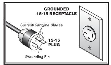
Figure 2. NEMA 15-15 plug and receptacle.
